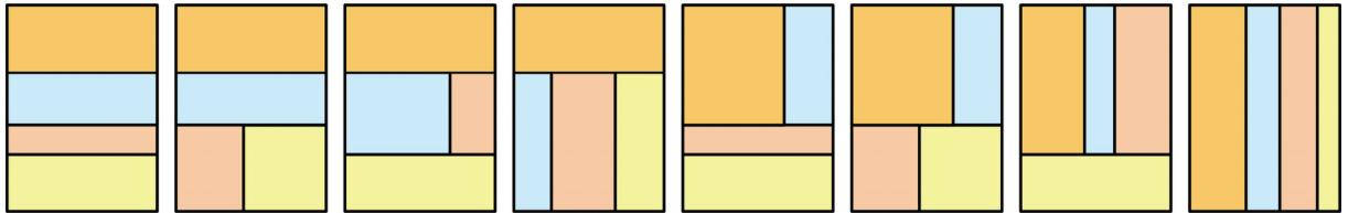
Figure 9: Eight possible ways to create four clusters for a given stripe
